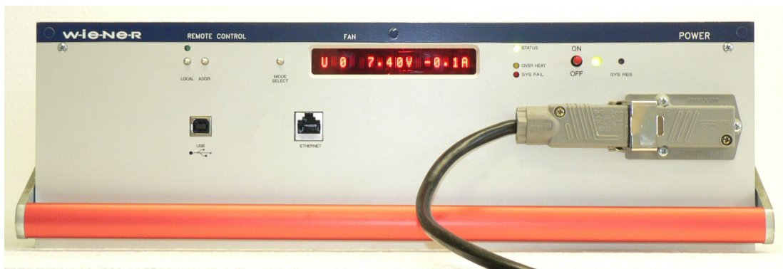
Figure 2.2: PL512/PL506 Front Side with Display Option
