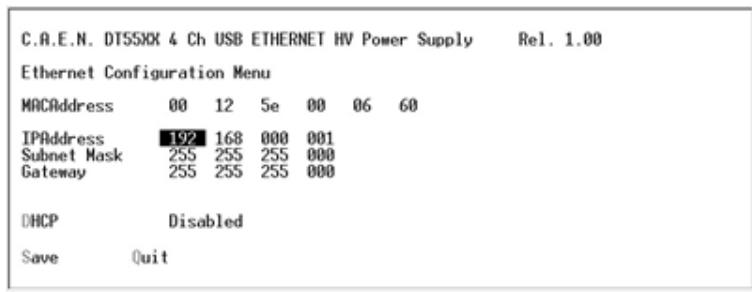
At first Power On the module is configured with default static IP (factory setting); such IP can be updated using the “arrows” to select the fields, typing the new values and confirming with <Enter>.
