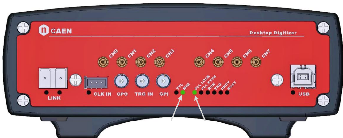
Fig. 13.1: Front panel LEDs status at power-on
