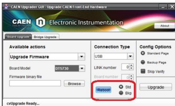
Fig. 14.1: Reboot section of CAENUpgrader
