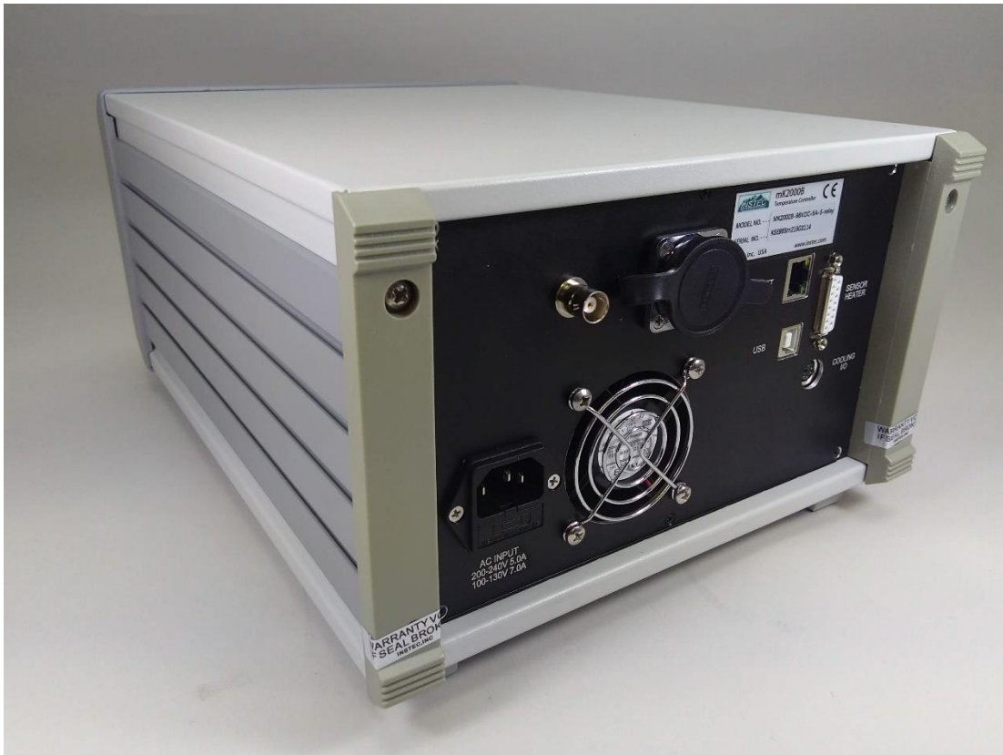
Figure 3. A sample The rear panel of the mk2000B controller (Nearly every mk2000B has a different rear-panel configuration). The serial number is unique for each controller, and the replacement fuse specifications are labeled under the fuse holder or on the nameplate/label.
