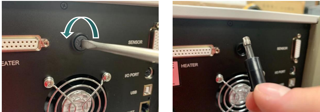
Figure A1: User replaceable AC Input Fuse Holder (left), and AC Input Fuse Drawer (right)
