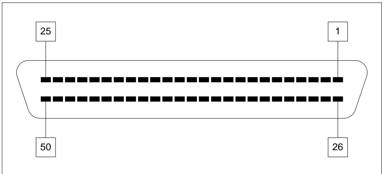
**Figure 4.1: Analog Output Connector**
